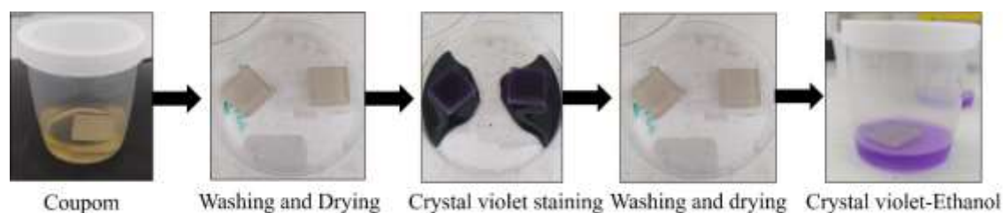
Figure 1 – Crystal violet assay: the coupons are soaked in Müller-Hinton broth, cleaned, stained, dried then placed in an ethanolic solution to determine absorbance
